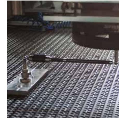
Calibración Ball Bar | Ball Bar calibration Calibration Système Ball Bar | Calibração sistema Ball Bar
