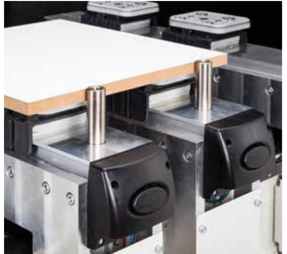
Easynest Evolution includes a revolutionary clamping system that combines the vacuum cup consoles and the multi-functional table for work in the Nesting system.
